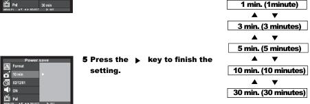
Only when using the batteries, the time for the auto power off function can be specified. When using the AC adapter (sold separately), the time for the auto power off function is fixed in 30 minutes and cannot be changed.
